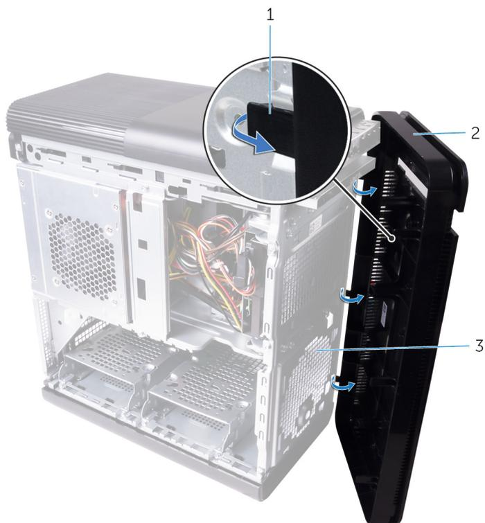
**Figura 6. Remover a tampa frontal**
