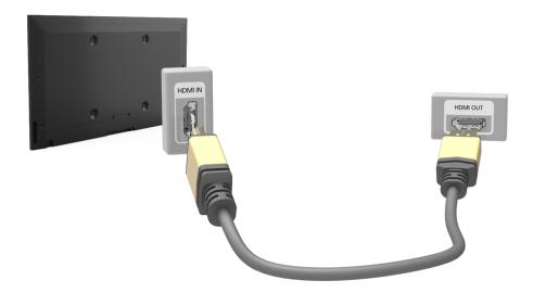
Once the connection has been made, you will be able to select the connected external device using the SOURCE button,
