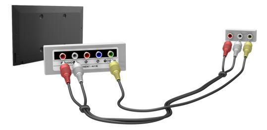
Once the connection has been made, you will be able to select the connected external device using the SOURCE button.
