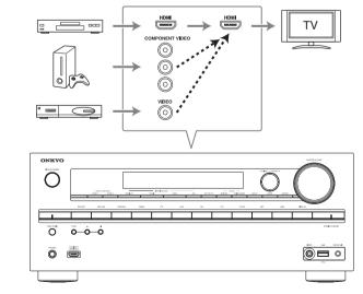
If you've connected your TV to the AV receiver with an HDMI cable, composite video and component video sources can be upconverted and output by the HDMI OUT MAIN.
